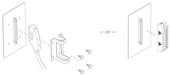
Use provided thumbscrews to secure cable or magnetic brick into 37-pin port. For right-angle cables ensure the cable exits down, for a magnetic brick the arrow should be visible on top. Secure cable with a metal bracket, a P-Clamp placed ~1 foot from 37-pin port, or both.
