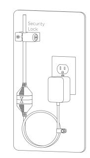
Connect magnetic cable directly to AC outlet and P-clamp double stranded coil.
