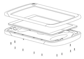
Connect your iPad to the included charging cable, and lay flat in the frame, slotting underneath the support in the top left corner. Seal with the front cover, flip over, and secure all provided screws.
