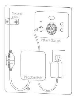
Install hub on headwall & connect to an AC outlet and patient station. P-Clamp wall side (short end) of magnetic cable.
