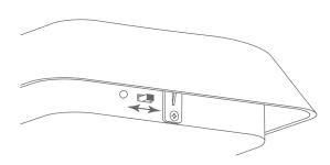
Certain PillowCase models are equipped with a physical UL1069 nurse call button in the top left corner, which will illuminate when powered and connected to a nurse call system. Pressing the button or disconnecting the magnet will place an emergency call, this can be disabled by moving the switch on the hub **away** from the LED.
