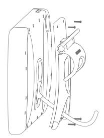
Align kickstand screwholes with central PillowCase screwholes and secure with provided longer screws.
