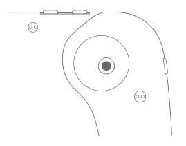
For optimal power & volume button performance, gently press & move the iPad to align the camera within the opening on the back **after** assembly.
